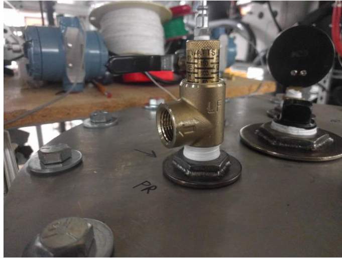
Figure 35: Pressure relief, set to 60 PSI
