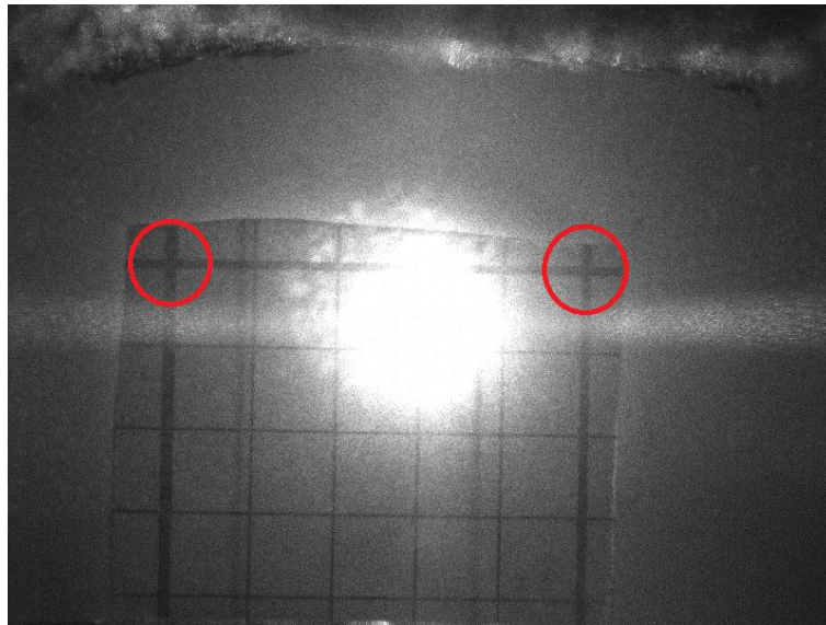
Figure 39: Pixel calibration using grid paper
