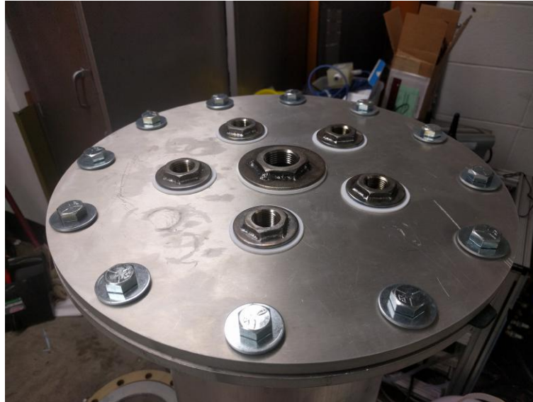
Figure 29: Top plate of pulse generator with bulkhead fittings attached
