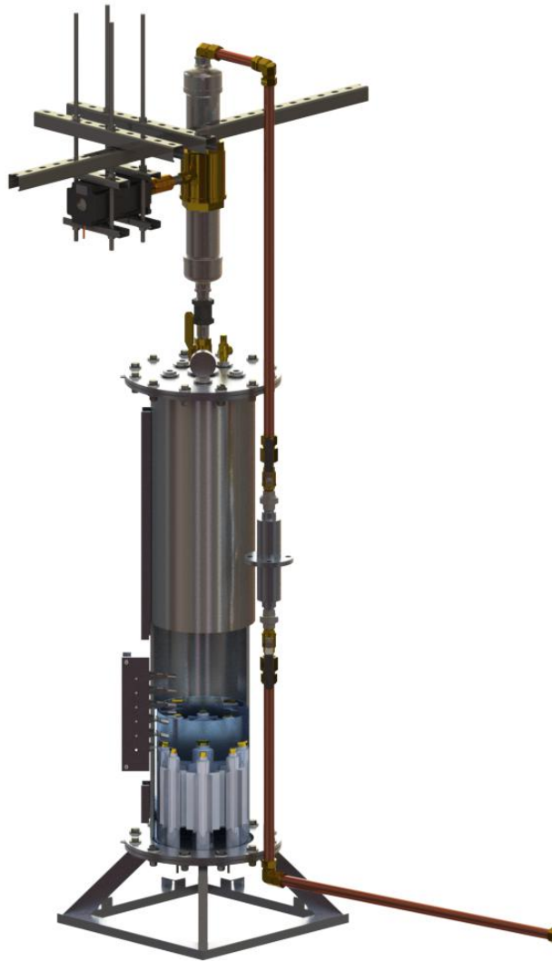
Figure 15: Cutaway rendering of the redesigned pulse generator installed in the MFVAL to copper plates, which were heated using chip resistors. The boiling refrigerant flowed back into the storage tank and increased the pressure inside the tank. After a sufficient pressure had been obtained inside the storage tank, a valve connected to the tank outlet was rotated using a stepper motor. Pulses of vapor would flow out of the pulse generator storage tank with each half-turn of the valve.
